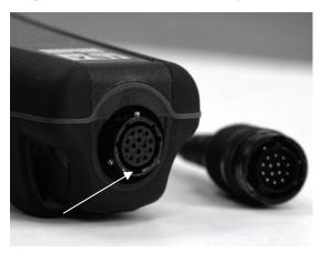
Figure 4, Note the keyed connector.
