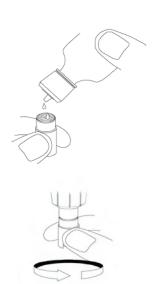
Fill a new membrane cap with  $O_2$  sensor solution that has been prepared according to the directions on the bottle. Be very careful not to touch the membrane surface.
